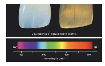
Depending on the type of crystallites, we get mean lengths of around 100 nm and 1,400 mm for lithium phosphate and lithium disilicate, respectively. This approximates the wavelength range of natural daylight and is responsible for the opalescence. Celtra thus behaves like natural tooth enamel in terms of light dispersion.
